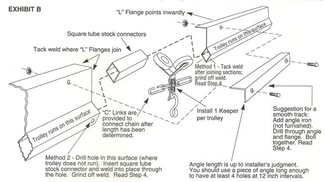
side of the track where a trolley wheel does NOT run. Insert a connector through the hole you drilled. Do this on all track sections (one hole only and one tack weld only per connection). Assemble all the sections. Grind off the tack weld at the holes.
